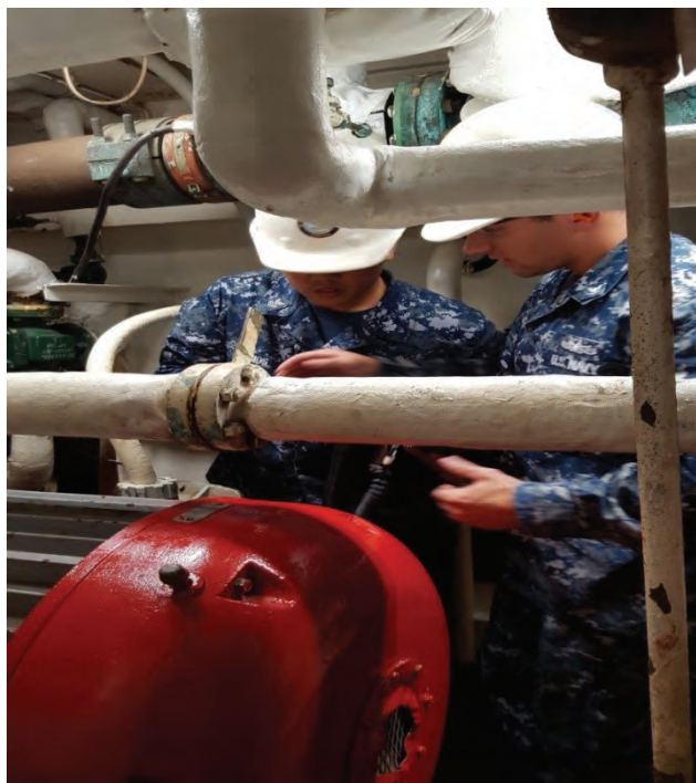
EM1 Christopher Ramos and EM3 Thomas Duca evaluating measured reading while conducting vibration analysis on NR6 Fire pump onboard USS Philippine Sea (CG 58).
