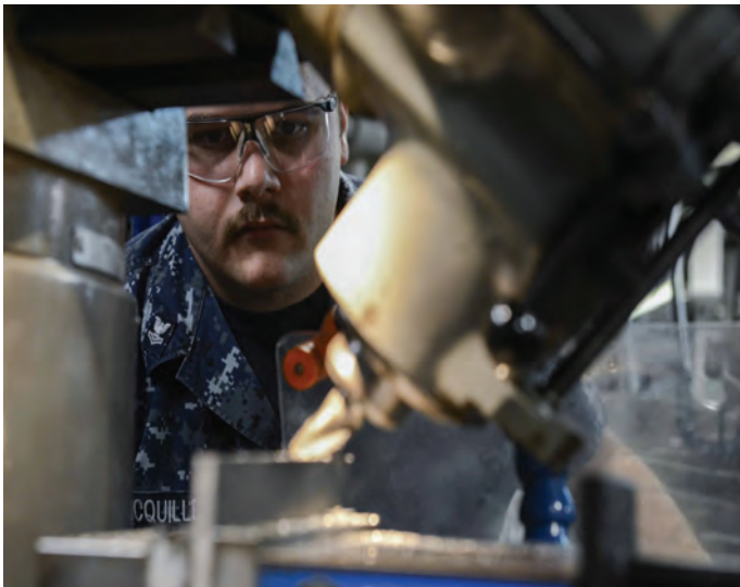
MR2 Timothy McQuillen, assigned to USS Nimitz (CVN 68), mills a 45 degree angle into a piece of bar stock.
