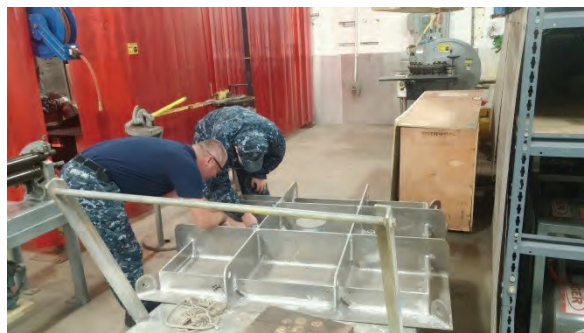
HT1(EXW) Jason Biberstine and HT1 Nolan Buford fabricating a cofferdam for SERMC Divers.
